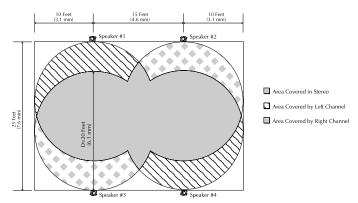
Figure 1 Stereo Coverage 4 speakers
